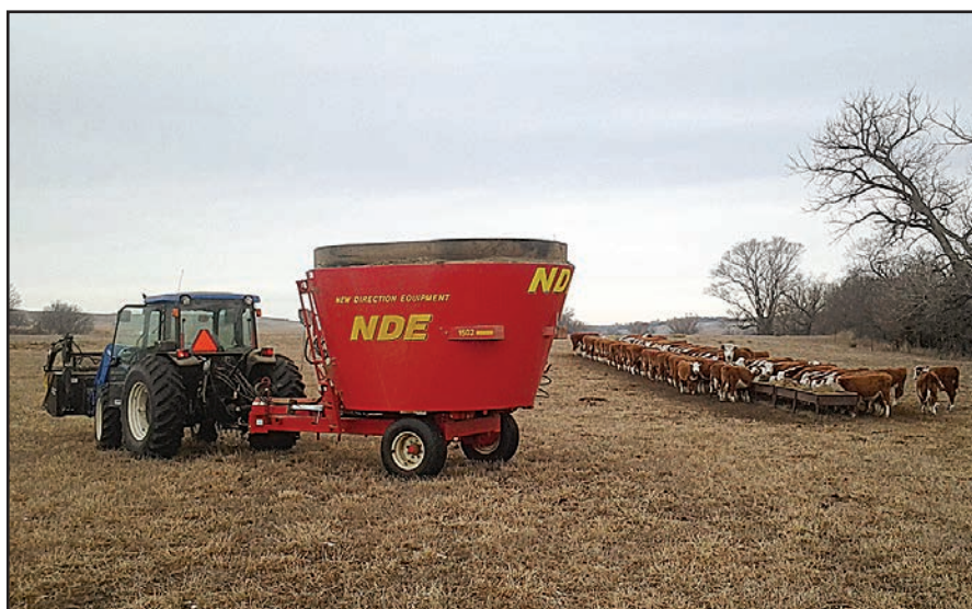
Hay Equipment 1 and 2 — Estermanns handle hay in bulk, using a big rake to help bring hay to the stack, a telehandler loader that can lift two tons onto the stack. Then hay is fed from a stack mover back to the cows. This last year they used a vertical mixing/grinding wagon to feed weaning calves.
